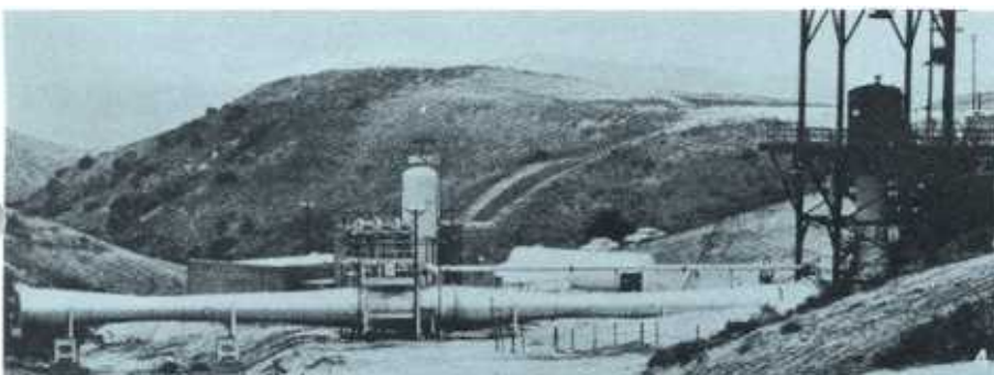
2. Three stage EVACTOR with Surface Condensers used in the continuous cooling of grain.
