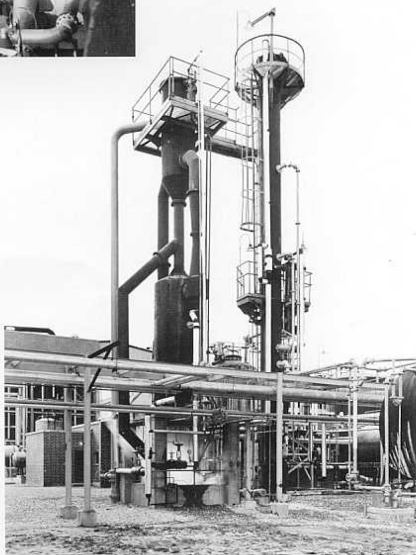
A two-stage self-supporting CHILL-VACTOR is installed in a paper-mill chlorine dioxide bleaching process.
