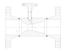
converging, stabilizing and diverging nozzle promotes the turbulent mixing of atomized water and steam thus maximizing efficiency in a wide range of process conditions including steady and variable flows.
