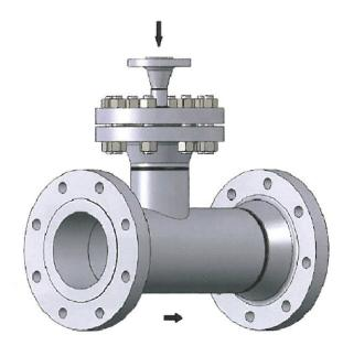
The venturi design, also known as an Attemperator, features a converging, stabilizing and diverging nozzle which promotes the turbulent mixing of atomized water and steam thus maximizing efficiency in a wide range of process conditions including steady and variable flows.
