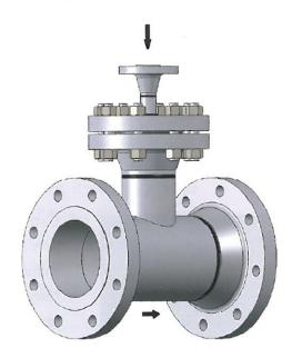
The Fixed Nozzle Desuperheater, also known as a mechanical desuperheater, is our most simple design. Water is introduced by way of a spray nozzle which creates a fine mist, thus cooling the superheated steam through the process of evaporation. The Fixed Nozzle design requires water pressure in excess of 5 bar (g) of the steam operating pressure.
