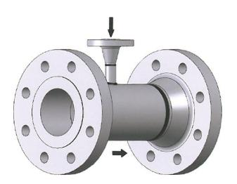
To complete its line of Venturi Desuperheaters, Croll Reynolds' Full Venturi Desuperheater features negligible pressure drop, offers a turndown ratio of 6:1 and is recommended when high pressure water and/or atomized steam is unavailable. This design will operate efficiently at low steam velocity and under conditions where the differential of water over steam pressure is 2 bar (g). The
